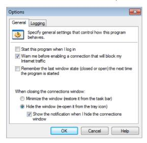
The General tab includes the following settings to control the launch of the Global VPN Client:
