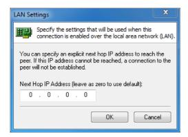
Type the IP address in the Next Hop IP Address field to specify the next hop IP address of a different route than the default route. Leaving the setting as zeros instructs the Global VPN Client to use the default route.
